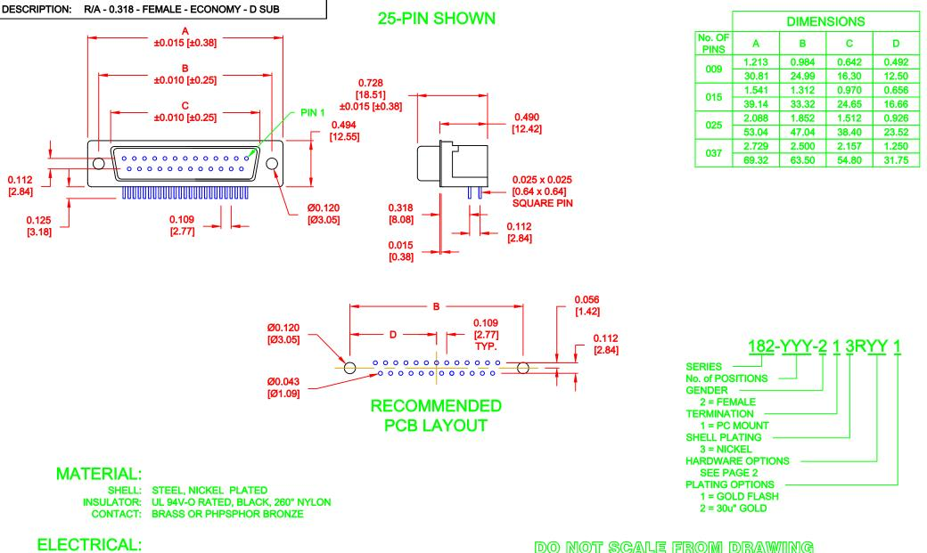
CURRENT RATING: 5 AMPS DIELECTRIC STRENGTH: 1,000VAC rms INSULATION RESISTANCE: 1,000 MOHMS Min
