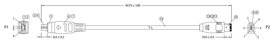
FRONT 1394 4P/M MOLDING TYPE (TOOLING NO.G102-288)
