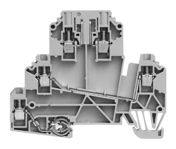
The new WDK 2.5 DU PE TR multiple level terminal blocks are designed to reduce cabinet space and increase functionality in signal-loop circuit installations. By connecting the signal wire to the upper level, the neutral to the lower level and the shield to the integrated PE contact, a signal loop can be connected to just one terminal.
