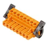
Socket connectors with clamping yoke screw connection for conductor connection with 270° outlet direction and release lever or release latch mechanism. The female connectors provide space for labelling and can be coded. Packed in cardboard box.
