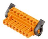
Socket connectors with clamping yoke screw connection for conductor connection with 270° outlet direction and release lever or release latch mechanism. The female connectors provide space for labelling and can be coded. Packed in cardboard box.br/>
