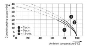
Derating curve for: PC 4/..-ST-7,62 with PCVK 4-7,62 DIN EN 61984 (VDE 0627):2002-09 Thermal test group C Derating curve, representation based on DIN EN 60512-5-2:2003-01 connected conductor cross section = 4 mm<sup>2</sup> Reduction factor = 0.8 No. of positions: See diagram Dimensioned drawing
