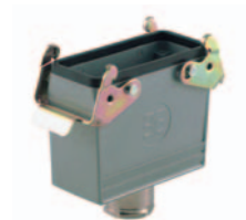
Top cable entry Without cover Side locking position With two locking levers High construction
