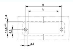
Dimension b = 10.84 mm + (no. of pos. x 5.08 mm) Dimension c = Dim. b + 5.83 mm
