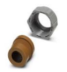
Half screw connection Pg21, made of plastic, consisting of rubber seal with one hole and one pressure screw, for type 2 - 4 housings, cable [mm] 9 - 13
