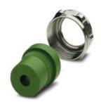
Half screw connection Pg16, made of metal, consisting of rubber seal with one hole and one pressure screw, for type 1 housings, cable [mm] 9 - 13
