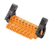
Female socket connectors with clamping-yoke screw system for connecting wires.
