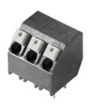
PCB terminal for fully automatic assembly in reflow soldering (SMT), with Push In conductor connection system. Conductor inserted and slider operated in same direction (TOP). Packed in box or as tape on reel. Pin lengths optimised at 1.5 mm or 3.5 mm.
