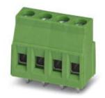
PC terminal block, Nominal current: 16 A, Nom. voltage: 400 V, Pitch: 5.08 mm, Number of positions: 4, Connection method: Screw connection, Mounting: Soldering, Conductor/PCB connection direction: 0 °, Color: green, The article can be aligned to create different nos. of positions!
