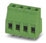
PC terminal block, Nominal current: 16 A, Nom. voltage: 400 V, Pitch: 5 mm, Number of positions: 4, Connection method: Screw connection, Mounting: Soldering, Conductor/PCB connection direction: 0 °, Color: green, The article can be aligned to create different nos. of positions!
