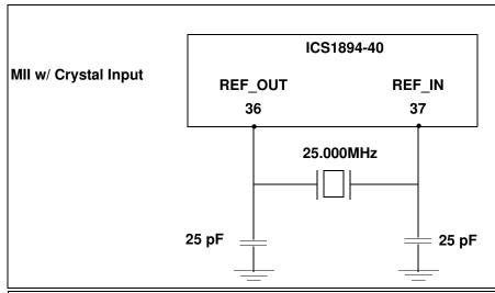
**NOTE:** 25 pF crystal load capacitors were required to bring the ppm for the 25 MHz crystal within the ±50 ppm on the IDT 1894 PHY evaluation board. The crystal used had a recommended load capacitance of 18 pF.
