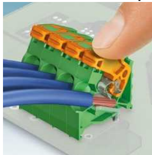
PLH 5 series: push-lock spring connection, 7.5 mm pitch, up to 41 A, connection: 30° to PCB PLH/A 5... Page 470
