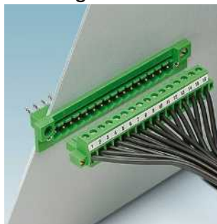
Headers for panel feed-through, 5.0/5.08 mm pitch, with spade connection DFK-MSTB 2,5/...-G(F)-... Page 352
