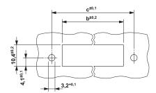
Dimension b: 10.49 mm + (no. of pos. x 5.08 mm) Dimension c: Dim. b + 9.27 mm
