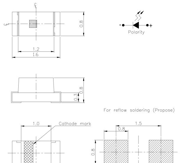
**Note:** The tolerances unless mentioned is  $\pm 0.1$ , Unit = mm
