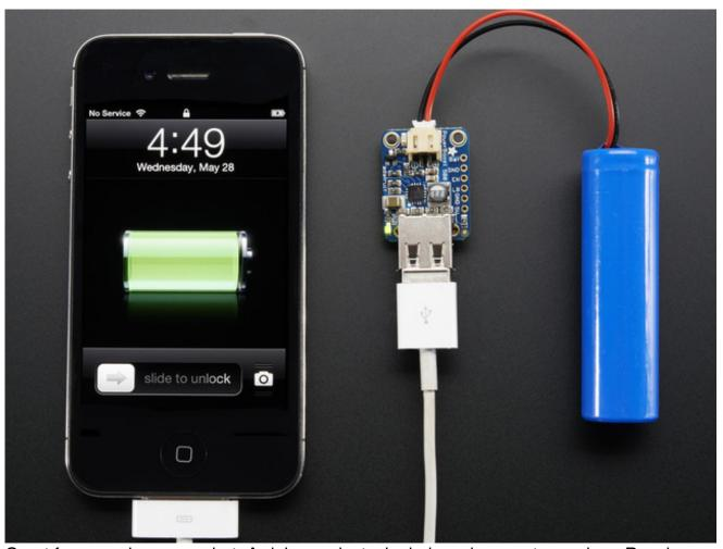
Great for powering your robot, Arduino project, single-board-computer such as Raspberry Pi or BeagleBone! Each order comes with one fully assembled and tested PCB and a loose USB A jack. If you are powering your project from USB, solder the USB A jack in (a 3-minute soldering task). If you would like to use a terminal block, pick up a 3.5mm 2pin block here (http://adafru.it/duR) and solder to the output spot where the USB jack would go. Or dont solder anything in for a more compact power pack.
