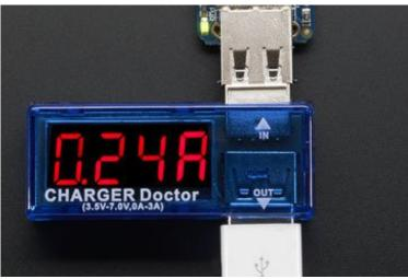
If you want to check the exact current draw during charge, try out a Charger Doctor between the USB port and charger. (http://adafru.it/dvm)
