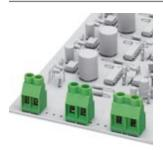
PCB terminal block, Nominal current: 32 A, Nom. voltage: 630 V, Pitch: 7.62 mm, Number of positions: 2, Connection method: Screw connection, Mounting: Soldering, Color: green, In order to avoid tolerances between the terminal blocks and the printed circuit board, they should be interrupted when the number of positions exceeds 30.
