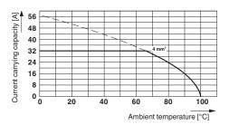
Type: MKDS 5 HV/2-9,52 and MKDS 5 HV/3-9,52 Test following DIN EN 60512-5-2:2003-01
