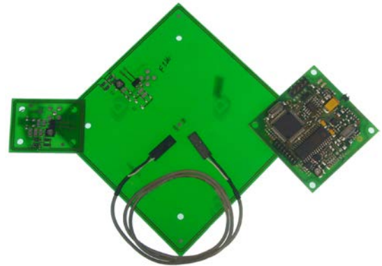
As external antennas, two 50Ω antennas ID ISC.ANT40/30 and ID ISC.ANT100/100 are available.
