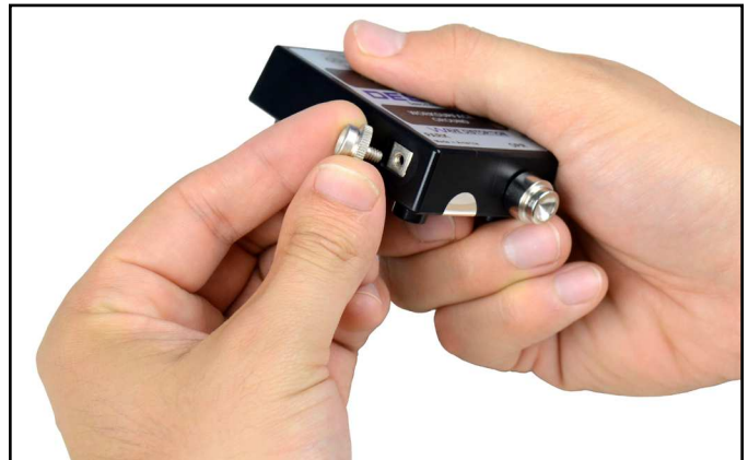
Figure 7. Changing the park snap on the 19243 Mini Monitor
