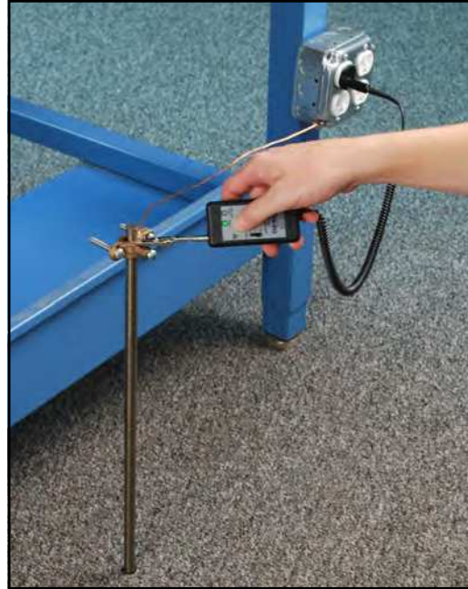
Figure 5. Testing auxiliary ground with the 19245 tester
