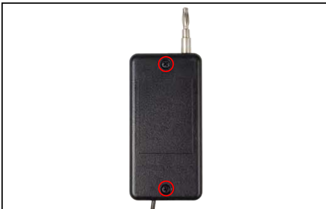
Figure 6. Locating the enclosure screws
