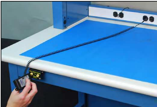
Figure 3. Testing ground points with the 19245 tester
