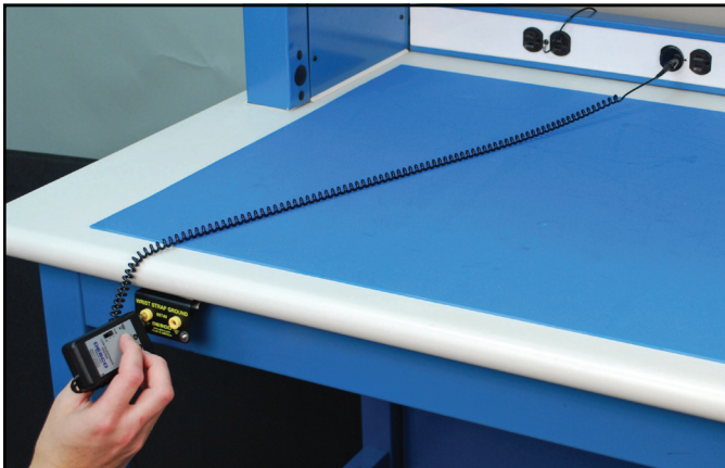
Figure 3. Testing ground points with the 19249 tester
