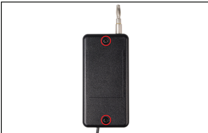
Figure 6. Locating the enclosure screws
