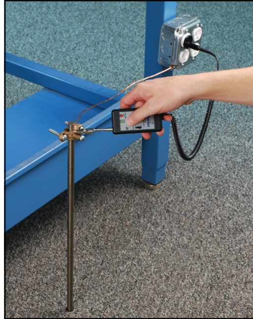
Figure 5. Testing auxiliary ground with the 19249 tester
