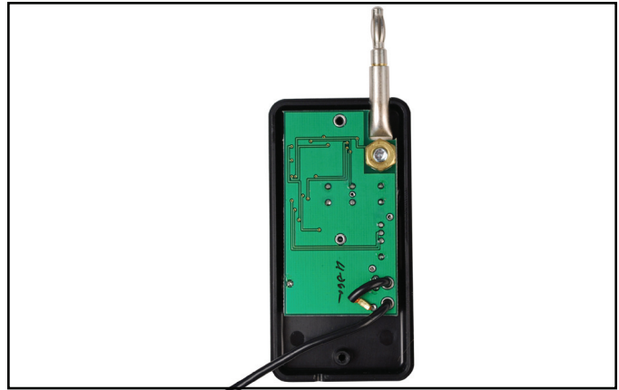
Figure 7. Removing the back cover
