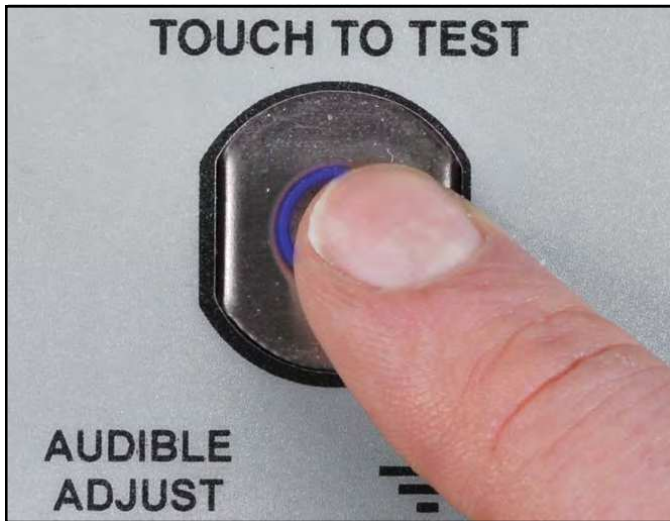
Figure 9. Bridging the test switch's contacts to initiate the test
