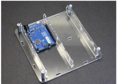
The horizontal braces now slot into notches on the verticals. Each of these is a different shape. The thinnest one is designed to clear the Arduino's power jack. The slightly thicker (but still pretty thin) brace goes down the middle, while the full-thickness one is at the bottom.
