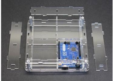
The four side pieces are almost identical...except for one which has a notch for the Arduino's USB port. Install this side first. Align the bottom tabs with the slots in the base and tilt it up into place. If the USB port is covered, you've got it backwards — turn it around and try again.
