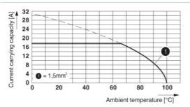
Derating diagram for 5 pins;reduction factor=1
