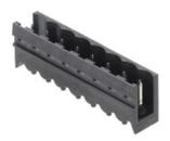
High-temperature-resistant, straight, open ended male connector. Packed in box or tape. In tape with 1.5 mm solder pin optimised for automatic assembly. 3.2 mm solder pin suitable for reflow and wave soldering. These male connectors can be labelled and coded.
