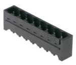
High-temperature-resistant male connector, packed in box or tape. In tape with 1.5 mm solder pin optimised for automatic assembly. 3.2 mm solder pin suitable for reflow and wave soldering. These male connectors can be labelled and coded. • 400 V (IEC) / 300 V (UL)
