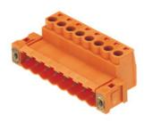
Male connector with screw clamping yoke connection for connecting conductors. The male connectors provide space for labelling and can be coded. Packed in cardboard box. • 0.20 - 2.5 mm<sup>2</sup> (IEC) / 26 - 12 AWG (UL)
