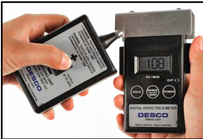
Figure 8. Taking decay measurements
