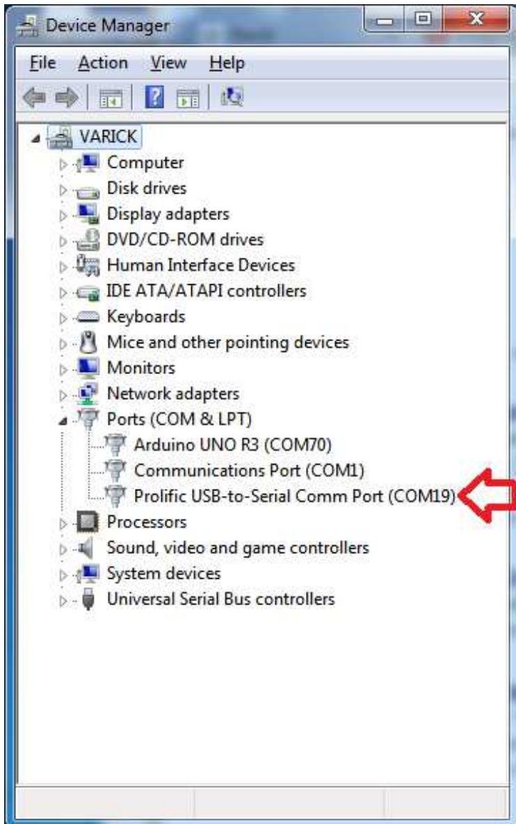
Connect to that COM port at 8N1 (8-bit, no parity bit, 1 stop bit) at 9600 baud. You can actually use any baud rate and it will autodetect but 9600 is supported by any terminal program!
