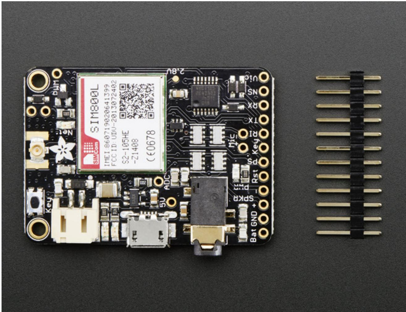
This module measures only 1.75" x 1.25" but packs a surprising amount of technology into its little frame. At the heart is a GSM cellular module (we use the latest SIM800) the size of a postage stamp. This module can do just about everything
