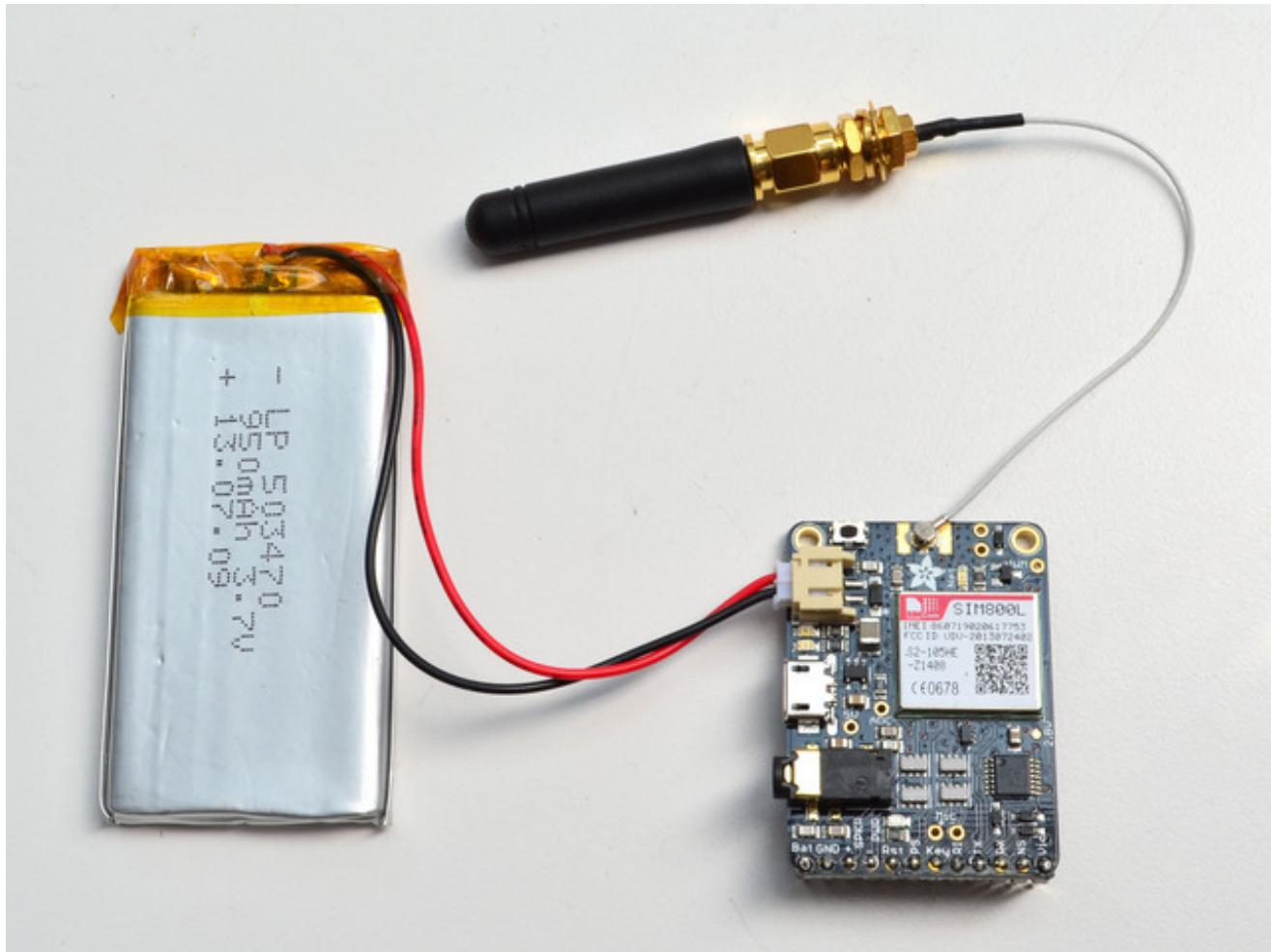
**Check polarity for the battery!**
