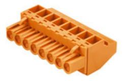
Socket connectors with clamping yoke screw connection for conductor connection with a right-angle (90° or 270°) outlet direction. The female connectors provide space for labelling and can be coded. Can be fastened with flange or release latch. They feature an integrated plus/minus screw, protection against false insertion under clamping yoke. They are delivered with an opened clamping yoke.
