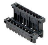
High-temperature resistant, double level, laterally offset, male connector with flange or solder flange. 1.5 mm solder pin is suitable for reflow soldering. 3.2 mm solder pin suitable for reflow and wave soldering. These male connectors can be labelled and coded. Packed in cardboard box.
