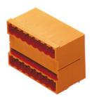
2-tier male connector with parallel pin arrangement. The solder pin length is optimised for wave flow soldering. The male connectors provide space for labelling and can be coded. Packed in cardboard box.
