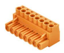
Female connectors with clamping yoke screw connection for conductor connection with straight (180°) outlet direction. The female connectors provide space for labelling and can be coded. Can be fastened with flange or release latch. They feature an integrated plus/minus screw, protection against false insertion under clamping yoke. They are delivered with an opened clamping yoke.
