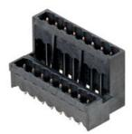
High-temperature resistant, double level, laterally offset, closed ended male connector, with solder flange option. 1.5 mm solder pin suitable for reflow soldering. 3.2 mm solder pin suitable for reflow and wave soldering. These male connectors can be labelled and coded. Packed in cardboard box. • 400 V (IEC) / 300 V (UL)
