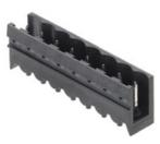
High-temperature-resistant, straight, open ended male connector. Packed in box or tape. In tape with 1.5 mm solder pin optimised for automatic assembly. 3.2 mm solder pin suitable for reflow and wave soldering. These male connectors can be labelled and coded. • 400 V (IEC) / 300 V (UL)
