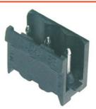
High-temperature-resistant male connector for side-by-side mounting. Packed in tape with 1.5 mm solder pin. Optimised for automatic assembly and suitable for reflow soldering. These male connectors can be labelled and coded.
