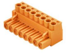
Female connectors with clamping yoke screw connection for conductor connection with straight (180°) outlet direction. The female connectors provide space for labelling and can be coded. Can be fastened with flange or release latch. They feature an integrated plus/minus screw, protection against false insertion under clamping yoke. They are delivered with an opened clamping yoke.
