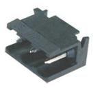
High-temperature-resistant male connector for side-by-side mounting. Packed in tape with 1.5 mm solder pin. Optimised for automatic assembly and suitable for reflow soldering. These male connectors can be labelled and coded.
