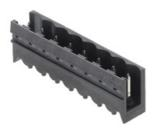
High-temperature-resistant, straight, open ended male connector. Packed in box or tape. In tape with 1.5 mm solder pin optimised for automatic assembly. 3.2 mm solder pin suitable for reflow and wave soldering. These male connectors can be labelled and coded.
