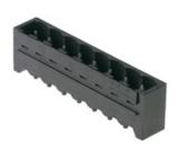
High-temperature-resistant male connector, packed in box or tape. In tape with 1.5 mm solder pin optimised for automatic assembly. 3.2 mm solder pin suitable for reflow and wave soldering. These male connectors can be labelled and coded.
