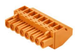
Socket connectors with clamping yoke screw connection for conductor connection with a right-angle (90° or 270°) outlet direction. The female connectors provide space for labelling and can be coded. Can be fastened with flange or release latch. They feature an integrated plus/minus screw, protection against false insertion under clamping yoke. They are delivered with an opened clamping yoke.
