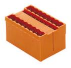
2-tier male connector with parallel pin arrangement. The solder pin length is optimised for wave flow soldering. The male connectors provide space for labelling and can be coded. Packed in cardboard box.
