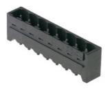
High-temperature-resistant male connector, packed in box or tape. In tape with 1.5 mm solder pin optimised for automatic assembly. 3.2 mm solder pin suitable for reflow and wave soldering. These male connectors can be labelled and coded. • 400 V (IEC) / 300 V (UL)
