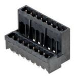
High-temperature resistant, double level, laterally offset, closed ended male connector, with solder flange option. 1.5 mm solder pin suitable for reflow soldering. 3.2 mm solder pin suitable for reflow and wave soldering. These male connectors can be labelled and coded. Packed in cardboard box.
