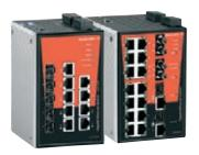
Weidmüller's Premium Line series completes the switch range for the high-end sector and is particularly suitable for complex network solutions with high traffic levels. The devices are available in different versions - number of ports, transmission rate (Fast and Gigabit Ethernet) and the type of connection (copper and fibre-optic).
