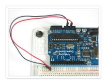
Now we'll provide power to the breadboard. Connect +5V to the red rail, and Ground to the blue rail.
