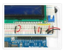
As mentioned, we'll not be using the **RW** pin, so we can tie it go ground. That's pin 5 as shown here.
