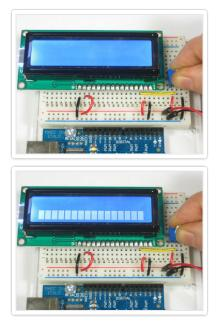
Now turn on the Arduino, you'll see the backlight light up (if there is one), and you can also twist the pot to see the first line of rectangles appear. This means you've got the logic, backlight and contrast all worked out. Don't keep going unless you've got this figured out!
