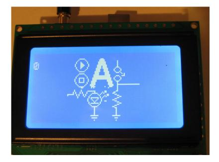
The graphical LCD has one big grid of pixels (in this case 128x64 of them) - It can display text but its best at displaying images. Graphical LCDs tend to be larger, more expensive, difficult to use and need many more pins because of the complexity added.
