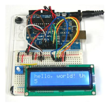
But the 20x4 LCD will 'wrap' the first line to the **third** line! (Likewise the 2nd line runs into the 4th) This seems really bizarre but its how the LCD memory configured on the inside. This probably should have been done differently but hey that's what we have to live with. Hopefully we'll have a future LCD library that is very smart and wraps lines but for now we are stuck. So when writing long lines to the LCD count your characters and make sure that you dont accidentally overrun the lines!
