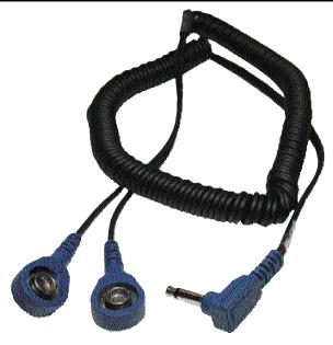
"If any part of the loop should open (become disconnected or have out of limit resistance), the circuit will go into the alarm state" [ref TR20.20], nonetheless, due to the redundancy inherent in the dual wire wrist strap design, the operator will continue to be grounded via the second intact wire.
