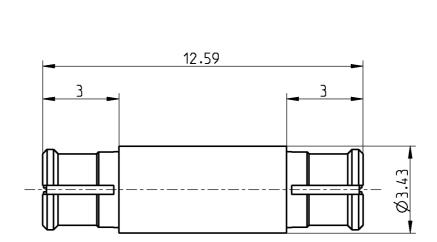
All dimensions are in mm; tolerances acc. ISO 2768 m-H
