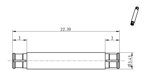
All dimensions are in mm; tolerances acc. ISO 2768 m-H
