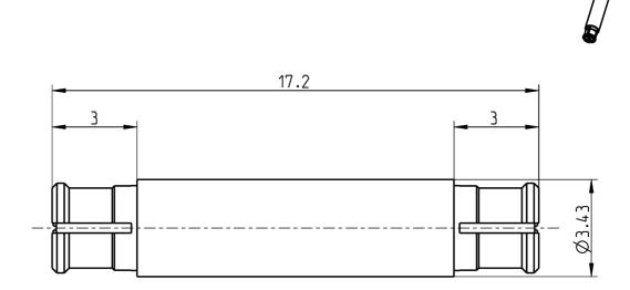
All dimensions are in mm; tolerances acc. ISO 2768 m-H
