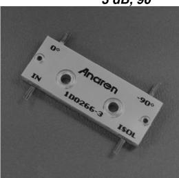
NOTES: Anaren Power rating applies when solder tab/coupler interface has been conformally coated.
