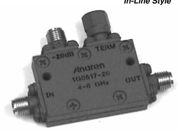
**NOTES**: The power rating applies when coupled port VSWR is 2.0:1 or less. Higher power can be handled with a lower VSWR termination Electrical and Mechanical Specifications subject to change without notice
