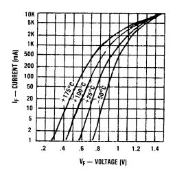
FIGURE 1 TYPICAL FORWARD VOLTAGE vs FORWARD CURRENT
